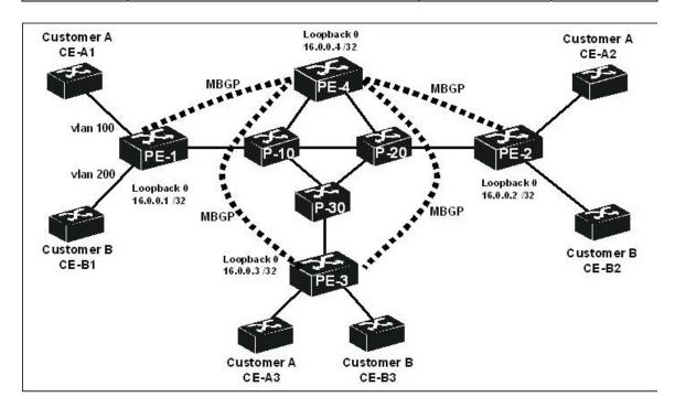
A provider of MPLS services configures MPLS Layer-3 VPN services for two customers. Each customer has three branch offices that will be interconnected. The address blocks chosen by the customers for each site are:
