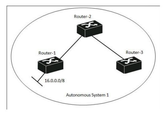
Router-1 and Router-2 are BGP peers. Router-2 and Router-3 are BGP peers. However, Router 3 has not learned the 16.0.0.0/8 BGP route. How can you resolve this issue? (Select two.)
