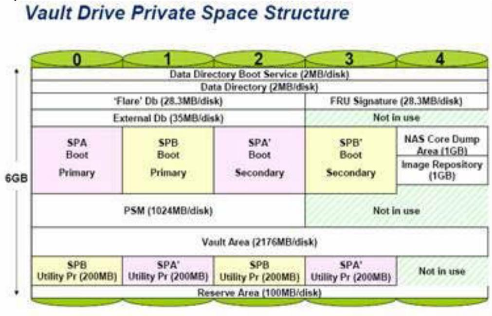
SP Boot Partitions - 2826.2 MB drives 0,1,2, & 3 - Each SP will have a mirrored SP boot partition. SPA will use drive 0 & 2 (0 is the primary with 2 as the mirror) and SPB will use drives 1 & 3 (1-primary, 3-mirror).
