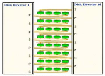
P = Primary Connection to Drive S= Secondary Connection for Redundancy
