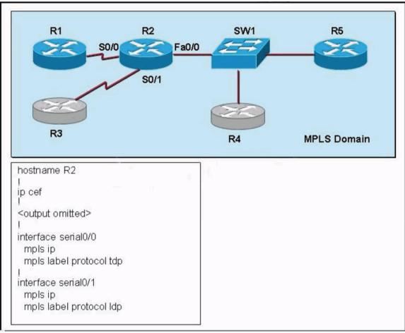
MPLS must be enabled on all routers in the MPLS domain that consists of Cisco routers and equipment of other vendors. What MPLS distribution protocol(s) should be used on router R2 Fast Ethernet interface Fa0/0 so that the Label Information Base (LIB) table is populated across the MPLS domain?
