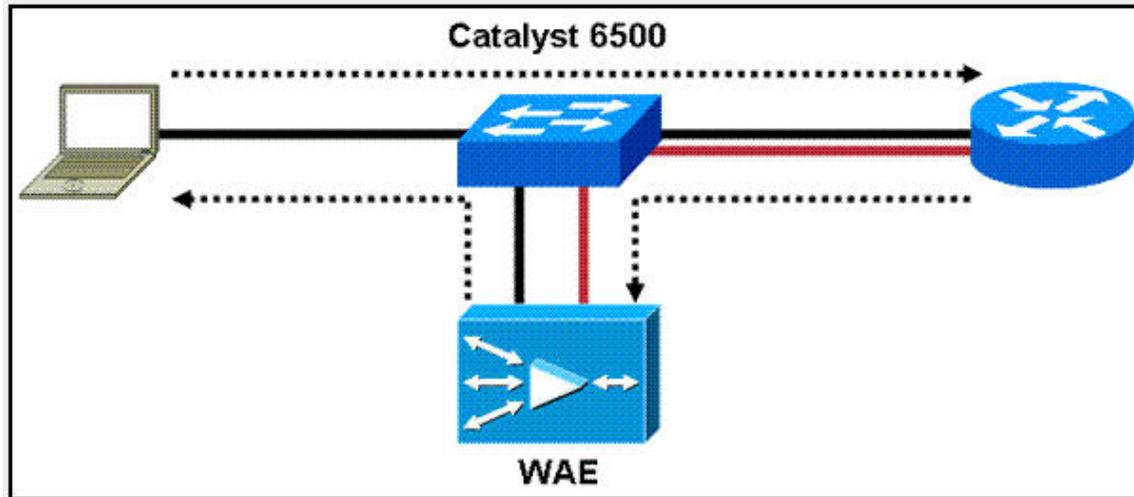
The WAE appliances are connected to Cisco Catalyst 6500 Series Switches and use WCCPv2 for traffic interception. The customer wants to minimize the latency added by interception. The customer also wants to know if Layer 2 redirection, rather than GRE tunnels, will improve performance.
