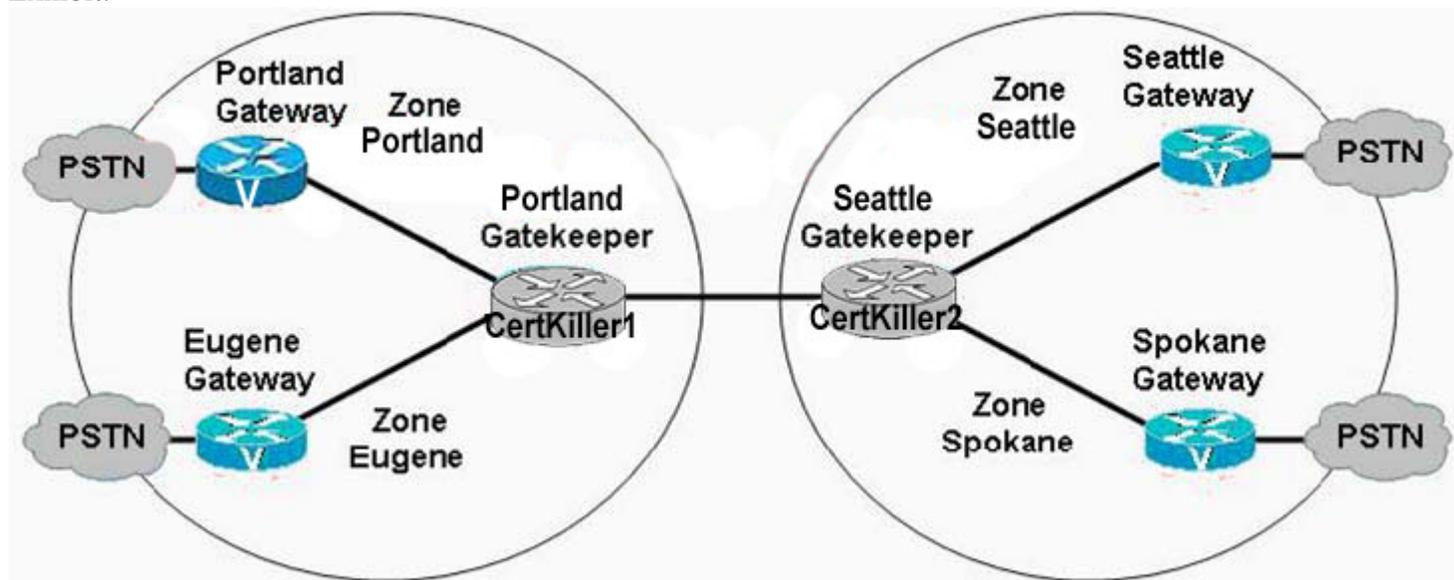
The network has two gatekeepers that control four zones. Which command is used to ensure that the aggregate bandwidth between zones that are controlled by the Portland Gatekeeper and the Seattle Gatekeeper is limited to 100,000 kbps?
