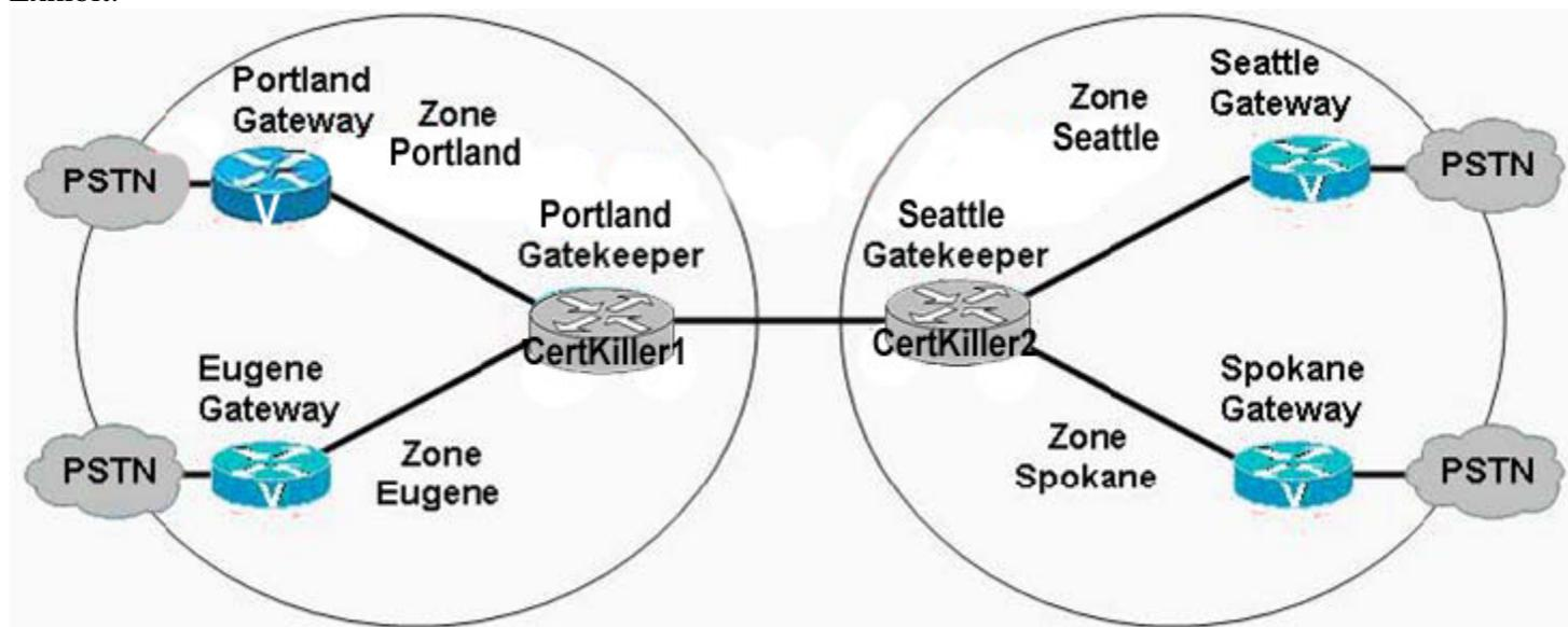
A network has two gatekeepers that control four zones. Which command is used to ensure that the aggregate bandwidth between the Seattle and Spokane zones is limited to 100,000 kbps?
