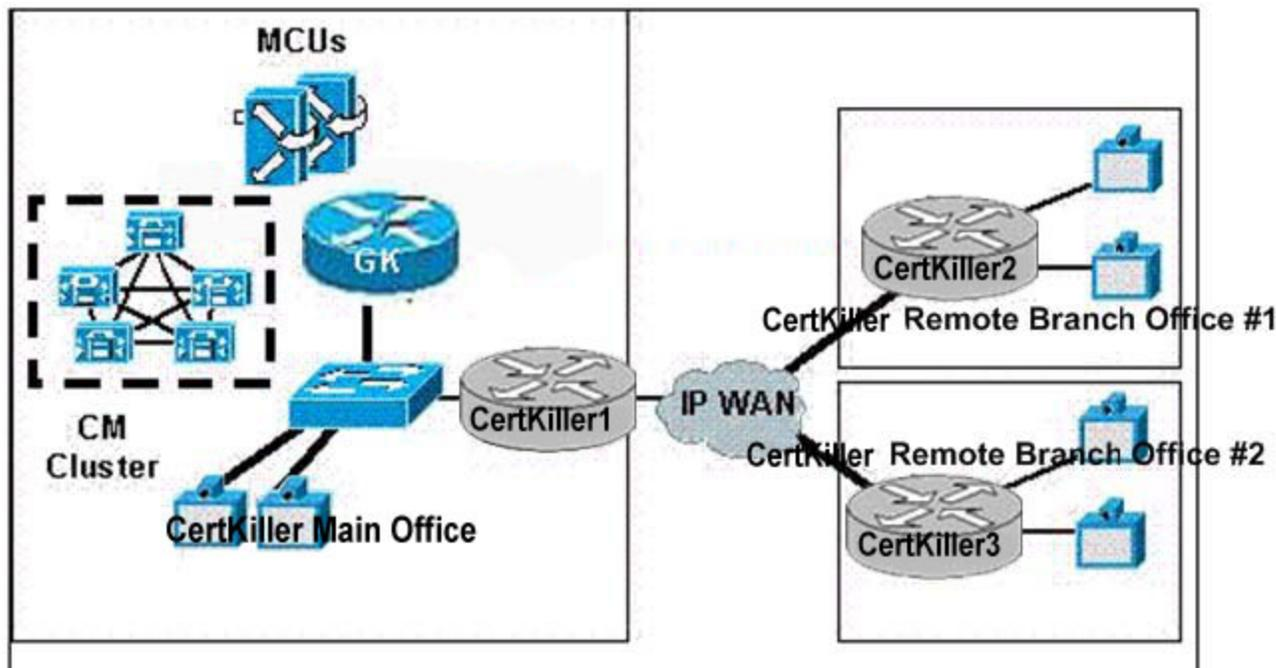
CAC is being configured for the centralized call-processing video telephony network. Each video terminal is capable of a maximum data rate of 320 kbps, and two video terminals are planned for each site. The requirement is to make two simultaneous video calls between the Certkiller main office and each remote Certkiller branch office site. The audio codec will be G.711. In order to ensure quality of service for calls, which action should be taken when configuring Cisco CallManager?
