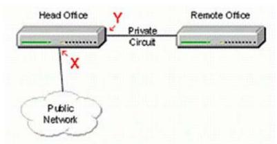
A customer has two sites, each with an IP Office linked via a private digital line (E1/T1). The head office is connected to the public network through a digital exchange line. The remote site gains access to the public network via the head office. How should Clock Quality be set in the IP Office on the lines marked X and Y in the exhibit?
